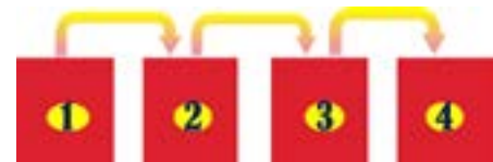
Cascading four power supplies
